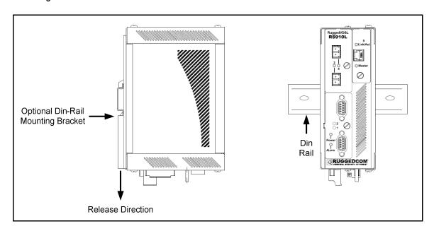
Figure 3 - RS910L DIN Rail Mounting
